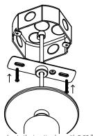
Mount the crossbar to the junction box with 8-32 flat head screws (provided).
