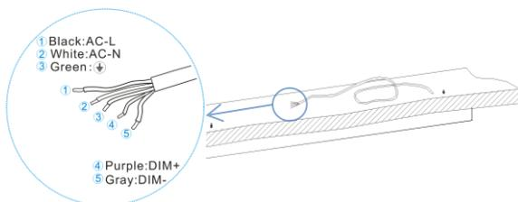
Explanation: connect to ①、②、③ only if do not need to use dimming function, no need to connect ④、⑤
