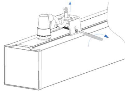
(5) Connect the lamp input line in outlet box according to the color mark corresponding to the city electricity and dimming signal line, strain relief device needs to be used before cord entry the outlet box during installation
