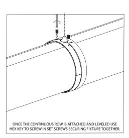
Fixture must be hung level at the desired height. If fixture is not level, light leaks may occur at the seam.
