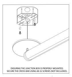
\*NOTE: JUNCTION BOXES MUST BE SOLIDLY FIXED TO THE CEILING AND ATTACHED TO THE STRUCTURAL MEMBER INSIDE THE CEILING BEFORE PROCEEDING WITH INSTALLATION.
