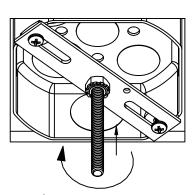
Thread the  $\frac{1}{4}\text{"-}20$  machine screw through the cross bar.
