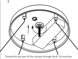
screw. Secure the canopy by using a  $\frac{1}{4}$ "-20 nut.
